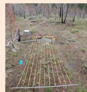
1. Average slope, ground cover, vegetation cover, and micro-topography were measured for each plot (all plots are 2x4 m).
