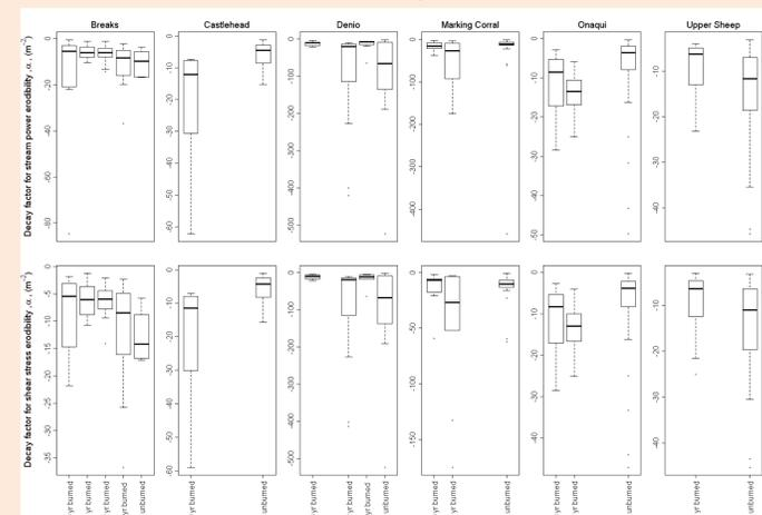
Decay factor ( $\alpha$ ) of stream power based concentrated flow erodibility, in  $K = K_{(Max)} \exp(\alpha q)$ , for all sites and treatments in this study.
