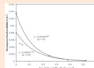
6. Values of  $K$  at each time step (i.e. time at which runoff samples were collected) within each flow release experiment was calculated (e.g.  $K_w = \frac{D_{cf}}{\omega}$ ). Then, the decay factor was calculated as the slope of the relationship between the values of log transformed  $K$  and the values of cumulative flow discharge ( $q$ ) to form the decay function:  $K = K_{(Max)} \exp(\alpha q)$ .
