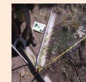
4. For each inflow rate, flow velocity was measured by salt tracer method while the width and depth of each flow path were measured by ruler at several transects.
