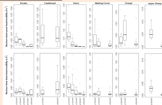
Maximum stream power concentrated flow erodibility coefficients calculated by  $K_w = \frac{D_{cf}}{\omega}$  and maximum soil shear stress concentrated flow erodibility coefficients calculated by  $K_s = \frac{D_{cf}}{\tau_s}$  for all sites and treatments in this study.
