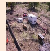
3. Water was released at different inflow rates approximately 4 m upslope of runoff collection point.
