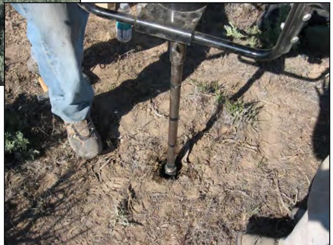
After the bar is fitted to the Auger and the Auger is fueled you can begin to operate. Generally, we take samples in 15cm increments: Mark the bit with a sharpie, at 15cm intervals before each sample. The measurements on the bar can be made using black electrical tape.
