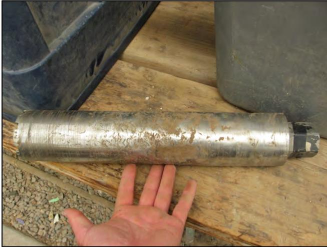
To the left is a close up of the bit, the indentations occur from striking the bit with a 3lb sledge to loosen the soil.
