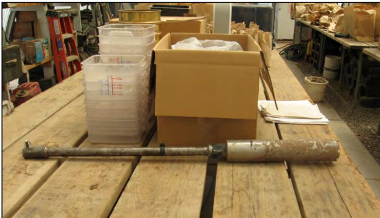
This photo shows both the custom made bar and the concrete bit. The bar can be purchased from a local machinist to fit your specifications. The concrete diamond bits are Ditec Supreme Pro core bits and cost between \$250-300. Each bit is good for 30-40 samples; depending on the type of material that is being cored.
